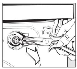
Using needle nose pliers, remove the plastic filter by pulling on the bar (see illustration). Rinse under water and return parts.
